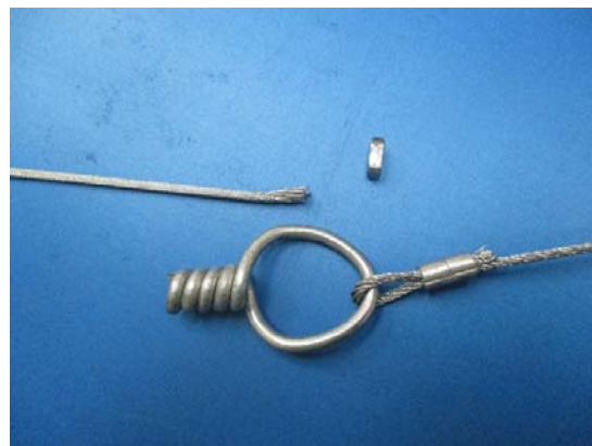
Test 3A – failure of centre swivel swage (note one clip and the washer were lost when the sample failed).
