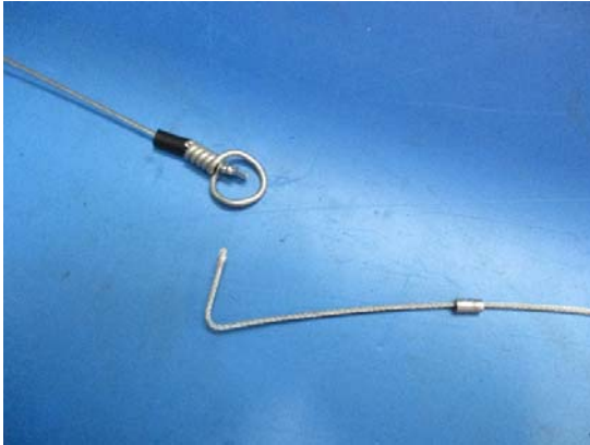
Test 1 – eye loop pulled out of swaged fitting at centre swivel
