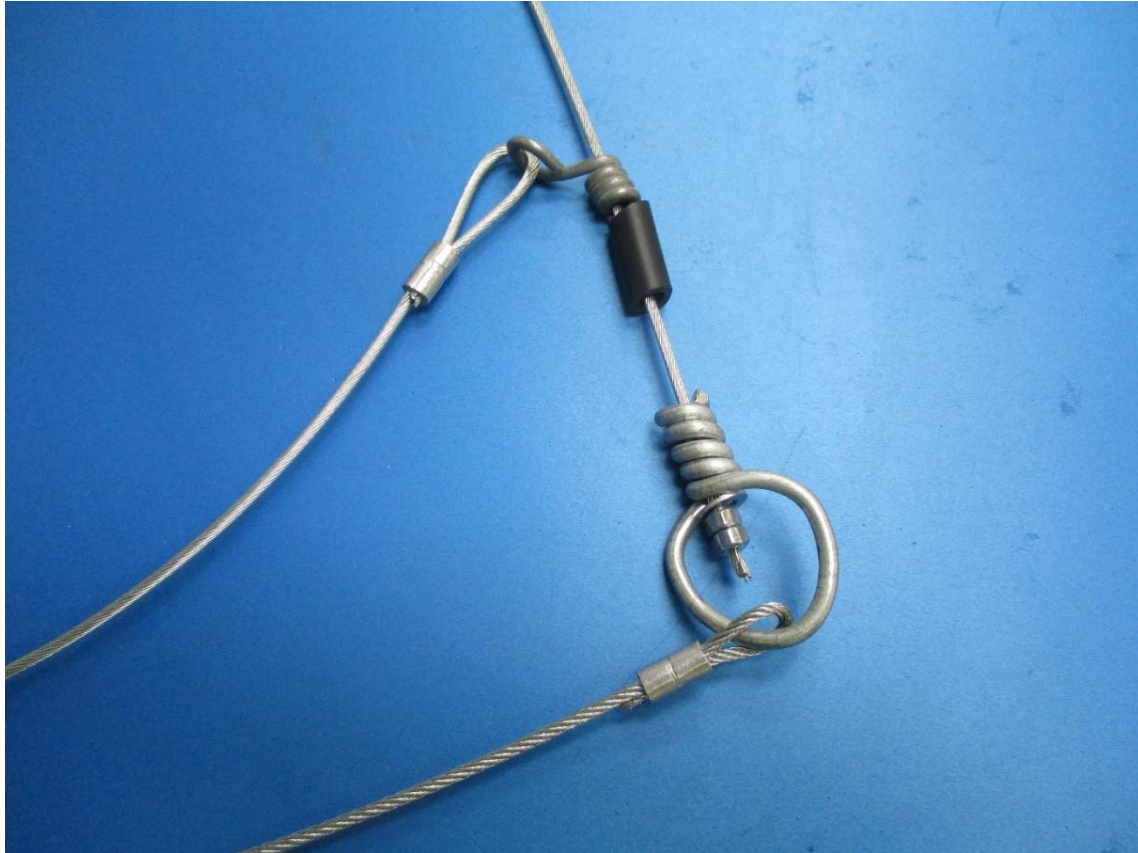
Figure 4.3: Detailed view on the centre swivel (middle right), and assumed breakaway weak link (top) on the sample supplied for testing. Note that the snare loop and lower securing section of wire rope are of different construction.
