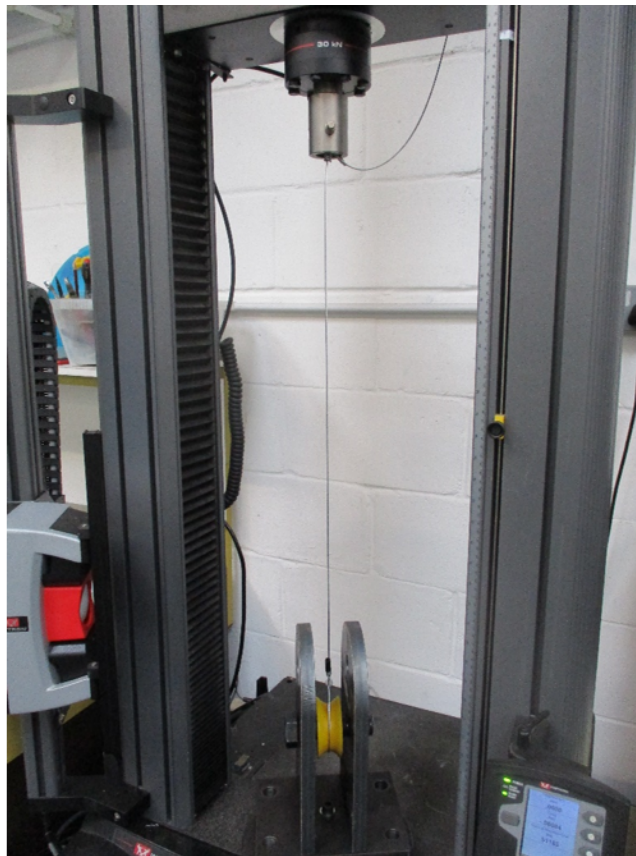
Figure 7.1: Showing the arrangement employed to test the sub-assembly strength (Test 3A). The bottom arrangement is as before and the swivel is mounted in the top fitting.
