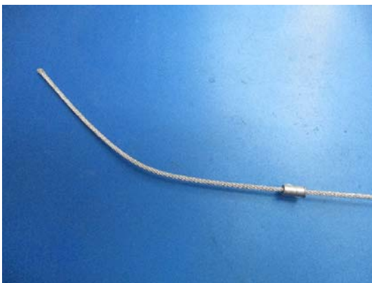
Test 3 – failure of ground eye loop swage
