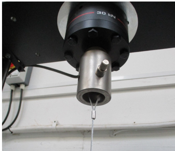
Figure 5.2: Ground eye loop mounted on the 30 kN load cell by \text{Ø}1/2 " steel pin.
