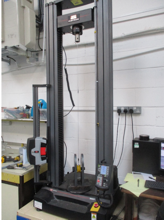
Figure 5.1: INSTRON tensile testing machine with breakaway snare mounted ready for testing.
