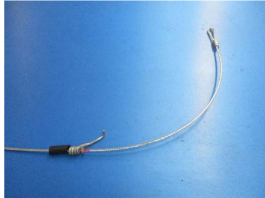
Test 1A – failure of weak link
